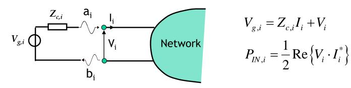
$$V_{g,i} = Z_{c,i}I_i + V_i$$
