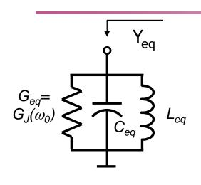
$$Y_{eq} = G_{eq} + j \left( \omega C_{eq} - \frac{1}{\omega L_{eq}} \right)$$
