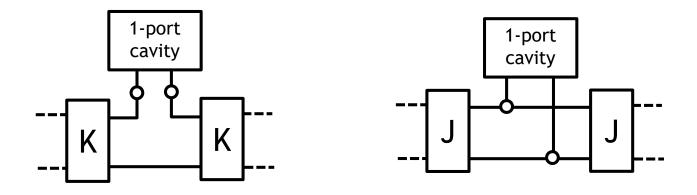
In case of 2-port cavities the equivalence should be imposed on all the elements of S or Z or Y matrix. It is however possible an approximation allowing to still refer to 1-port resonator
