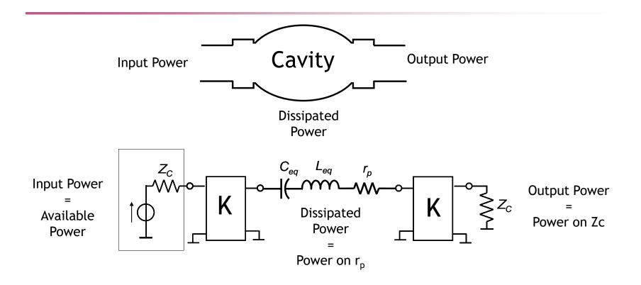
$$A_{dB} = -10\log\left(1 - \frac{2Q_L}{Q_0}\right) \cong 20\log\left(1 + \frac{Q_L}{Q_0}\right) \quad \left(Q_0 >> Q_L\right)$$
