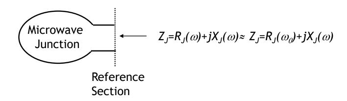
**Goal:** model of the junction in a defined frequency range B around  $f_0$  (B<< $f_0$ )
