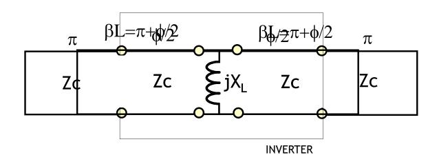
$$\beta L = \pi + \frac{\phi}{2} = \pi - \tan^{-1}(2X_L) \qquad X_L = \frac{K}{1 - \left(\frac{K}{Z_C}\right)^2} \approx K \quad (\text{for } K << Z_C)$$
