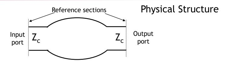
Given a physical structure, the <u>Scattering Parameters</u> (S matrix) allow a representation of its behavior in terms of the waves propagating on the transmission lines that connect the structure with the external world. Each line is characterized by its characteristic impedance  $(Z_c)$ , the phase velocity (v) and a reference section (defined port) at which the structure is observed.
