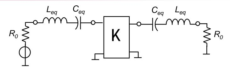
$$\omega_0 L_{eq} >> R_0 \implies \text{Input/output coupling } \approx 0$$
