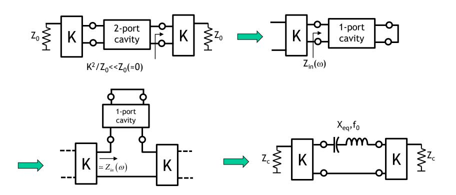
In general, this is acceptable for narrowband filters ( $B/f_0$ <<1), but represents a further approximation that is added to the approximation of the cavity with a lumped resonator
