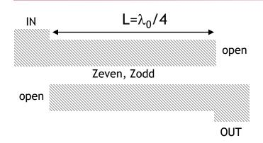
$$\omega_0 L_{eq} = \frac{1}{2} \omega_0 \frac{\partial X_S}{\partial \omega} \bigg|_{\omega = \omega_0} = \frac{\pi}{4} Z_m$$
