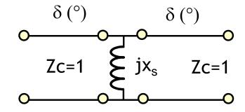
Equivalent circuit (reference sections: symmetry axis)
