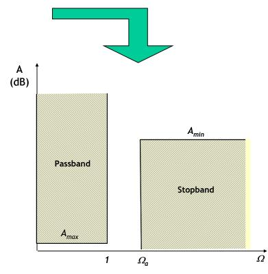
$$\Omega_{a} = \frac{f_{0}}{B} \left( \frac{f_{s,1}}{f_{0}} - \frac{f_{0}}{f_{s,1}} \right), \quad A_{\min} = A_{\min 1}$$
