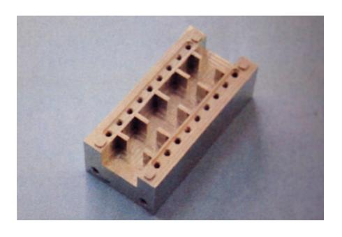
Example of fabricated device (4 resonators sample)
