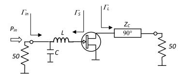
The transistor has the following parameters:  $S_{11}=0.6987 \angle -66.5^{\circ}$   $S_{21}=12.315 \angle 126.8^{\circ}$   $S_{12}=0.0474 \angle 57.3^{\circ}$   $S_{22}=0.7908 \angle -33.5^{\circ}$
