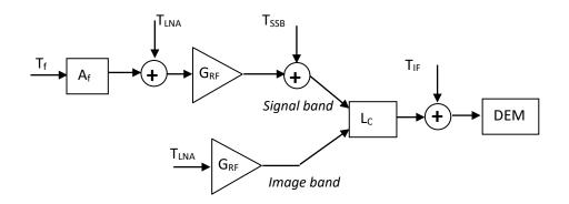
The equivalent noise temperature reported at the input is given by:
