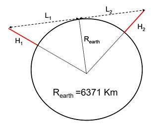
The maximum length is limited by the Earth's surface curvature.
