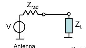
If the antenna is pointed in the direction of the incident wave and  $Z_L = (Z_{rad})^*$ :
