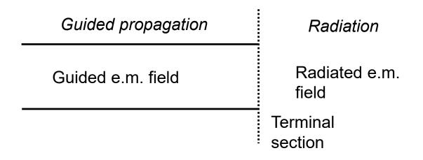
• The terminal section is a transition between guided propagation and radiation
