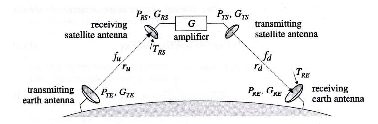
$f_u$ =Up-link frequency (6 GHz), *fd*=Down-link frequency (4 GHz) r<sub>u</sub>, r<sub>d</sub>>36000 Km (depends on the angle beneath which the satellite is seen) G<sub>TE</sub>, G<sub>RS</sub>, G<sub>TS</sub>, G<sub>RE</sub>= Gain of earth and satellite antennas P<sub>TE</sub>, P<sub>TS</sub>=Transmitting powers (earth and satellite) G = Gain of satellite transponder
