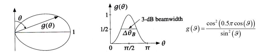
• The parameter  $\Delta \vartheta_{B} = \vartheta_{3dB}$  is called *half-power beamwidth* and is defined by the two values of  $\vartheta$  where g is halved with respect the direction of maximum
