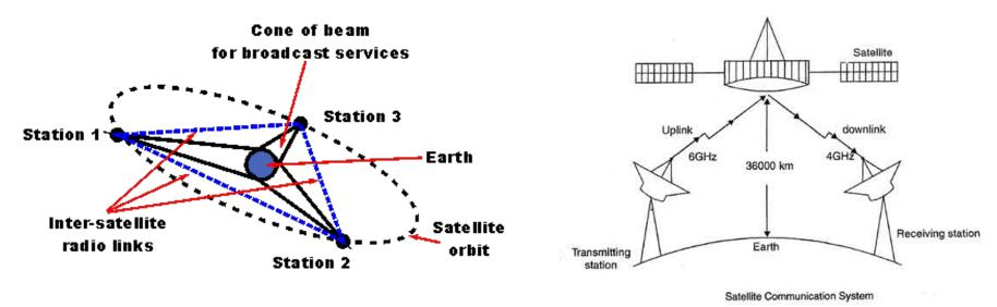
A geostationary satellite rotates in the same direction as the rotation of the Earth and has an approximate 24 hour period. This means that it remains in the same position relative to the Earth.
