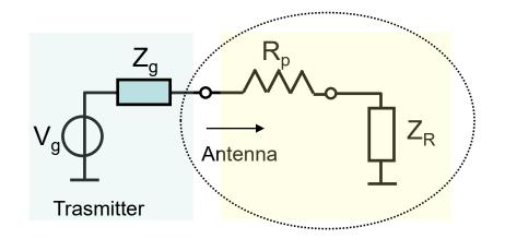
The impedance "seen" by the transmitter is determined by two contributions:  $Z_R$  (<u>radiation</u> <u>impedance</u>) and  $R_p$  (<u>loss resistance</u>). The power dissipated by  $Z_R$  constitutes the radiated power. Typically  $R_p <<|Z_R|$
