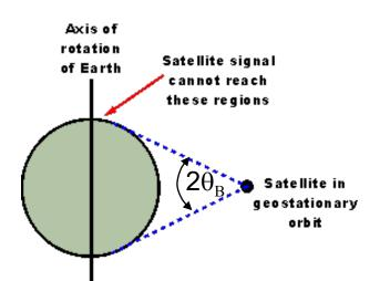
The value of  $\theta_{\rm B}$  is obtained by imposing the distance of geo satellite (~36000 Km) and the earth's radius (6371 Km). We get:  $2\theta_{\rm B}$ =17.36°
