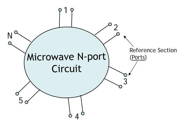
A microwave linear circuit is constituted by the interconnection of lumped and distributed elements. The interaction with the outer is realized through the <u>external ports</u>, which are defined on transmission lines outgoing from the network.
