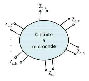
For a linear circuit, incident and reflected waves are linearly related:
