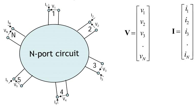
Assuming the network linear, the superposition principle allows the evaluation of the voltages at the ports, for a given vector of imposed currents (or vice versa). The matrices Z and Y are then introduced:
