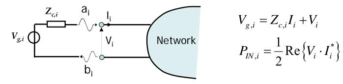
$$V_{g,i} = Z_{c,i}I_i + V_i$$
