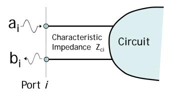
(1/2)  $|a_i|^2$ : Incident power wave = Available power from a source with impedance  $Z_{ci}$
