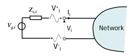
$$egin{aligned} V_i &= V_i^+ + V_i^-, & I_i &= I_i^+ + I_i^- \ V_i^+ &= Z_{c,i}I_i^+, & V_i^- &= -Z_{c,i}I_i^- \end{aligned}$$
