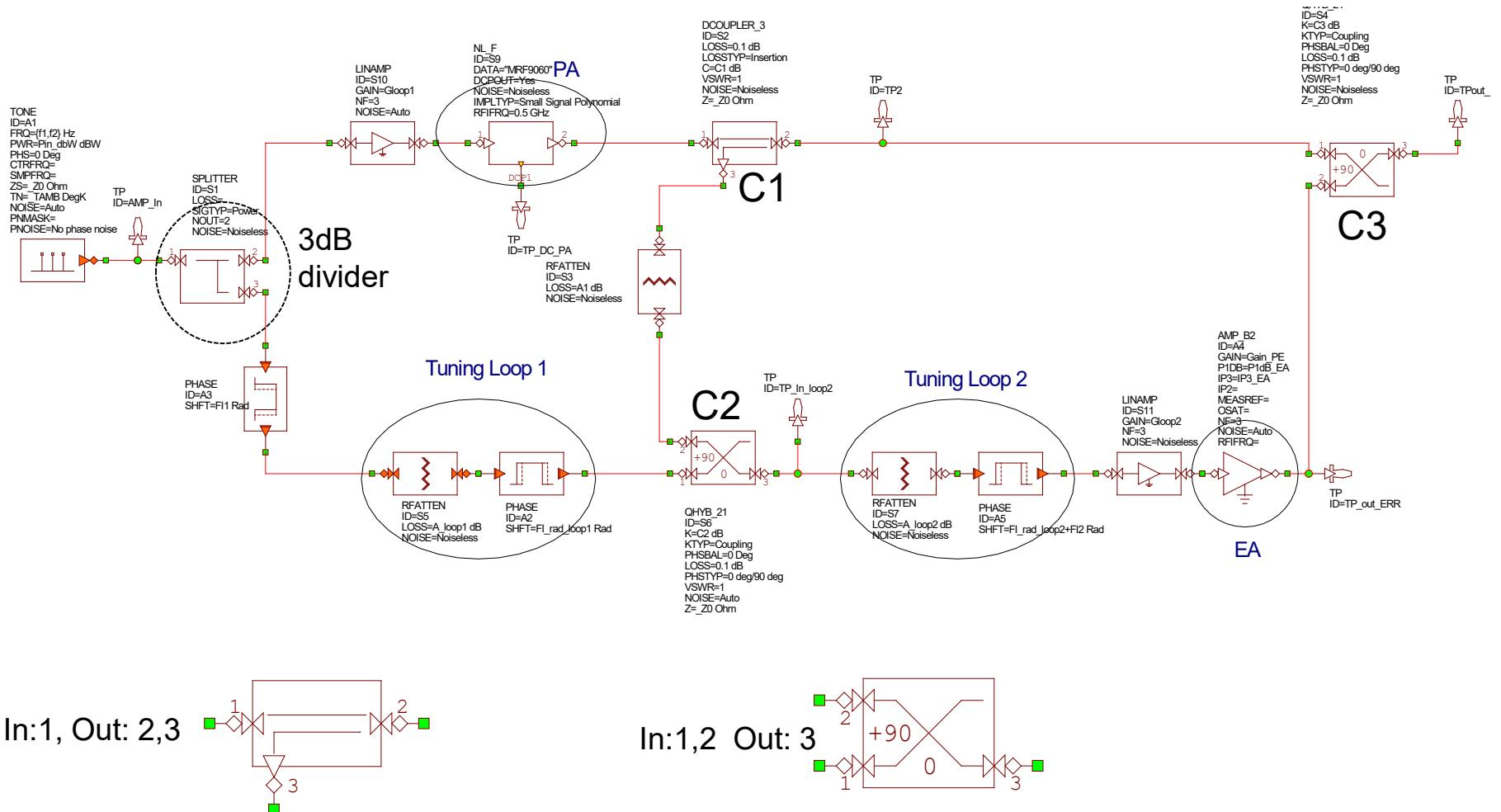
$$S_{21} = \sqrt{1 - 10^{\frac{C_{db}}{10}}}, \quad S_{31} = j10^{\frac{C_{db}}{20}}$$
