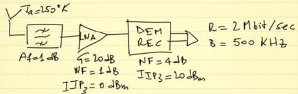
With the received signal equal to the receiver sensitivity, the  $E_b/N_0$  at baseband is equal to 15 dB.
