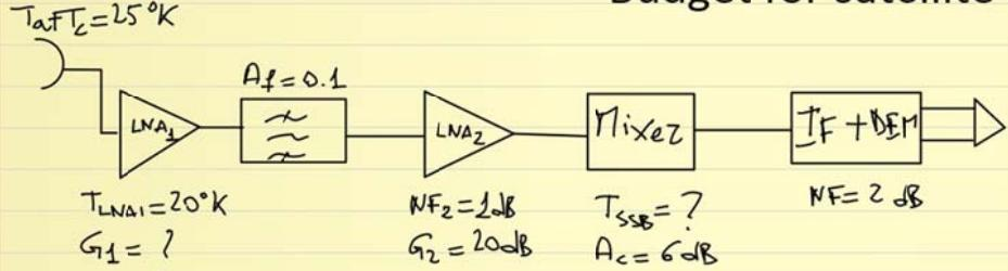
This figure represents the frontend of a receiver for a satellite ground station.
