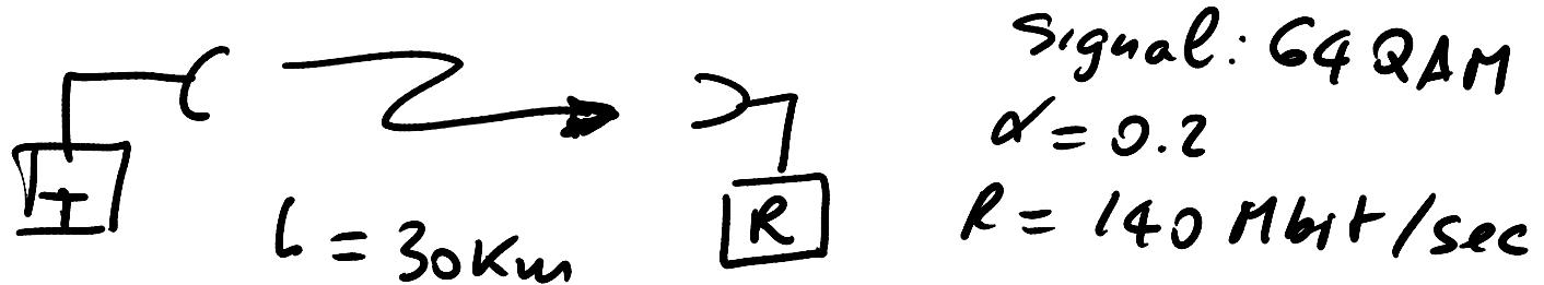
Antennas:  $G_T = G_R = 30 \text{ dB}$ ,  $T_a = 200^\circ\text{K}$
