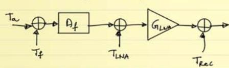
$$\begin{aligned} T_a &= 250 \text{ K} \\ T_f &= 290 (10^{0.1}) = 75.1 \text{ K} \\ T_{LNA} &= 75.1 \text{ K} \\ T_{REC} &= 290 (10^{0.4}) = 4384 \text{ K} \end{aligned}$$
