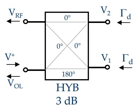
$$V_2 = \frac{V^+}{\sqrt{2}}, \quad V_1 = -\frac{V^+}{\sqrt{2}}$$
