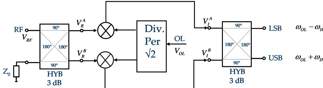
$$V_{OL} = V_0 \cos(\omega_0 t), \quad V_{RF} = V_U \cos((\omega_0 + \omega_{IF})t) + V_L \cos((\omega_0 - \omega_{IF})t)$$
