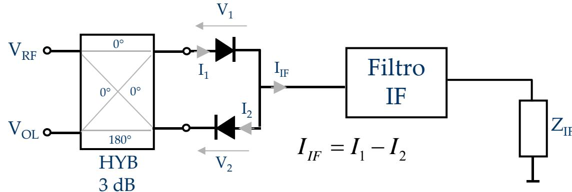
I/V characteristic of diodes:  $I_D = a_1 V_D + a_2 V_D^2 + a_3 V_D^3 + \dots$
