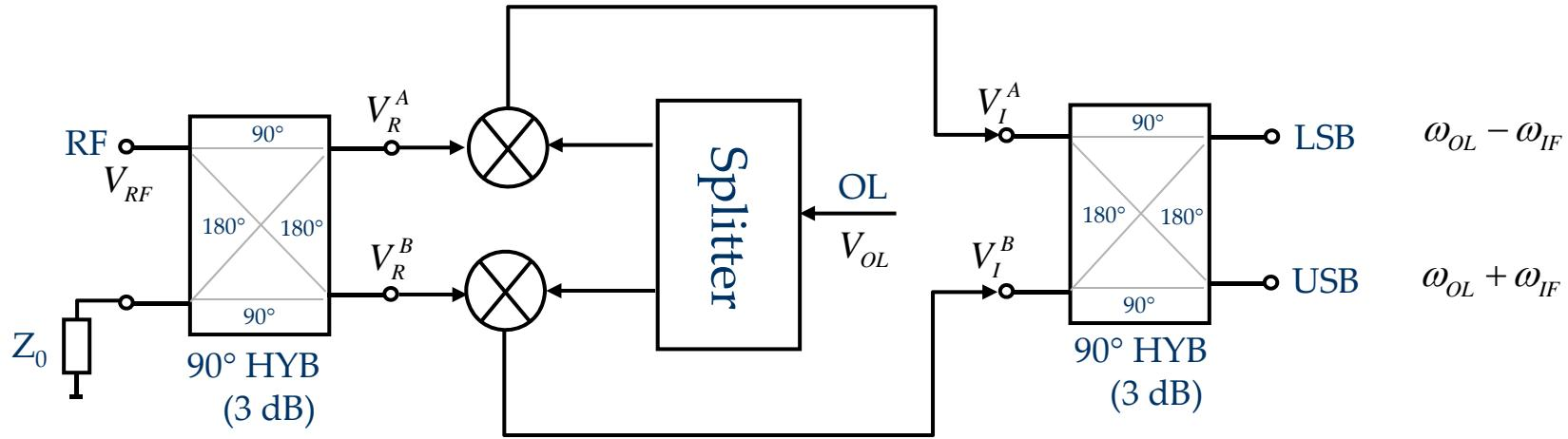
This configuration separates the translated and image signals. The image filter is then no more necessary (or its requirements are strongly reduced)
