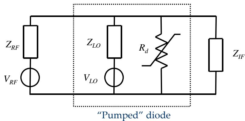
The diode ( $R_d$ ) is represented by the exponential curve:
